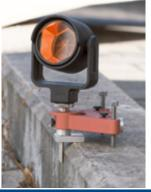
**C.4**. Ball prism bases for industrial 3D-Measurements
