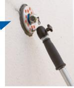
CONE: Cone adapter for measuring bolts and boreholes D.4.
