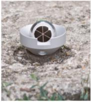
In the example shown here, the axis pin has been left out, since the ball prism can also be inserted without the cone adapter axis pin.
