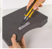
Cut out grid foam using cutter / parcel knife. Tip: Use a sharp knife. Do not "tear" but cut.
